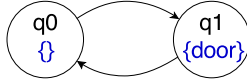
Fig. 1: Transition system \mathcal{T}_e for an environment with one door, which is initially open and can close or reopen at any time thereafter (there are implicit self-loops on each state). Here \mathcal{E} = \{q_0, q_1\} , \mathcal{E}_0 = \{q_0\} , \rightarrow = \{(q_0, q_0), (q_0, q_1), (q_1, q_0), (q_1, q_1)\} , \mathcal{L}_e(q_0) = \{\} , and \mathcal{L}_e(q_1) = \{\text{door}\}
